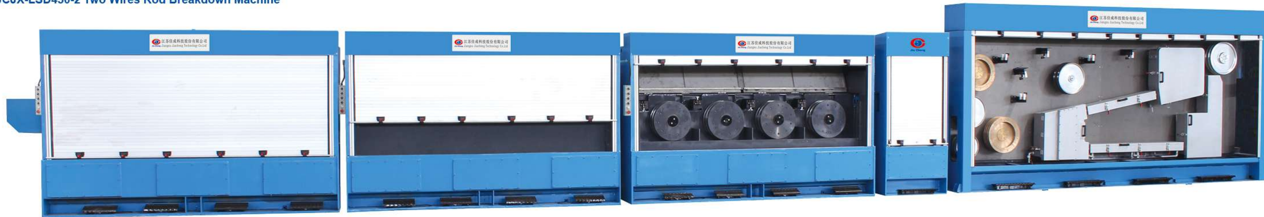
JCJX-LSD450-2 型双头微滑式大拉机 JCJX-LSD450-2 Two Wires Rod Breakdown Machine
